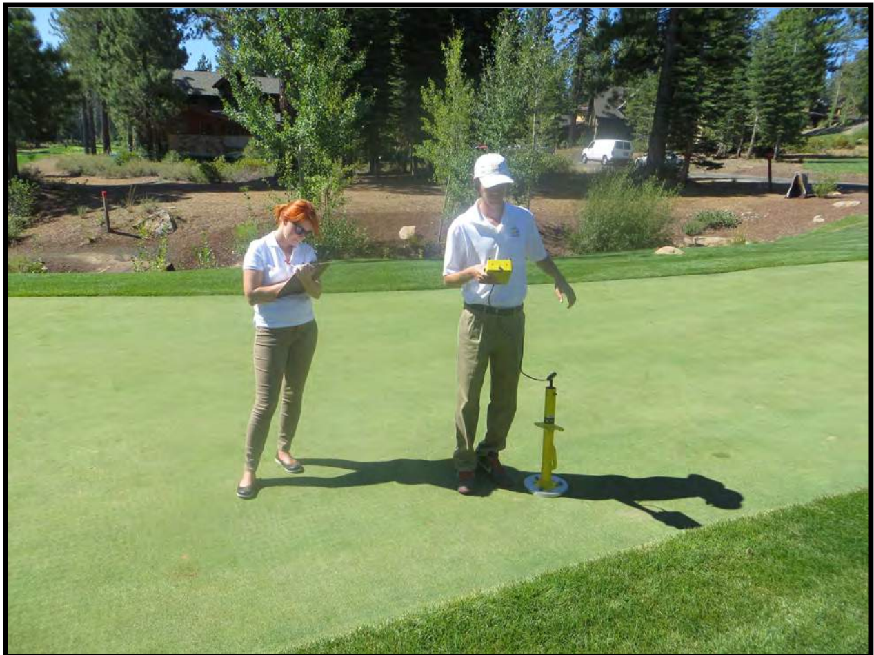
Figure 2. Study area on the 10th Putting Park green at Martis Camp Club, Truckee, CA. Photo was taken on 12 August 2013, the final rating date for the study. Similar to the USGA TruFirm instrument, the Clegg Impact Tester (shown here) provides a measurement of surface firmness.
